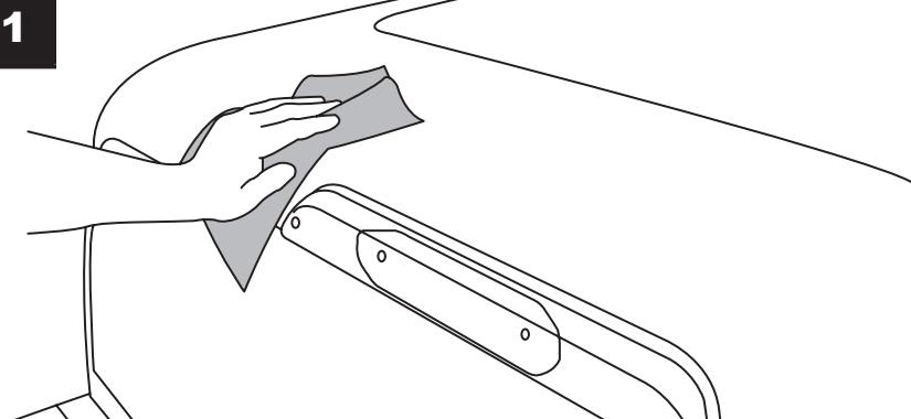
EN Clean the area of the roof where the spoiler will be in contact with the surface using only soap & water and dry with a clean cloth.
