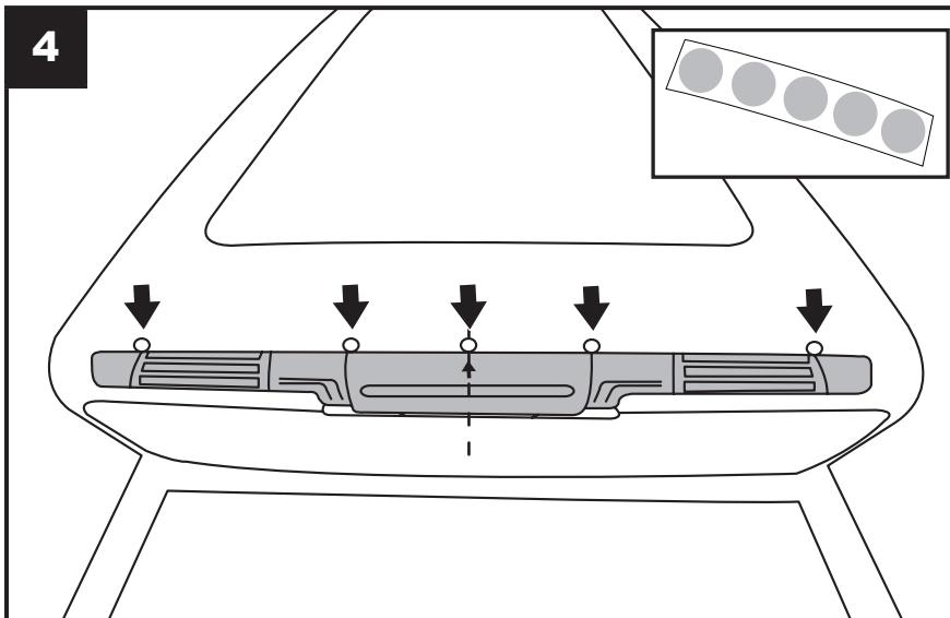
EN While applying pressure on the spoiler, install the 5 alignment stickers to the front edge of the spoiler to mark locations. Starting at the center, aligned with the spoiler's arrow.
