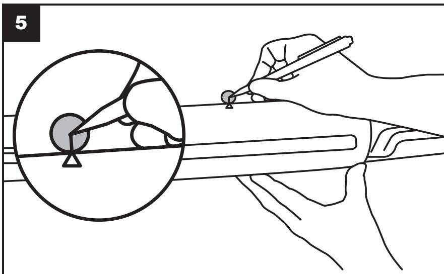
EN While applying pressure on the spoiler, pencil in, a line on the central alignment sticker in line with the arrow at the center of the spoiler to ensure its ultimate reference location during final installation.
