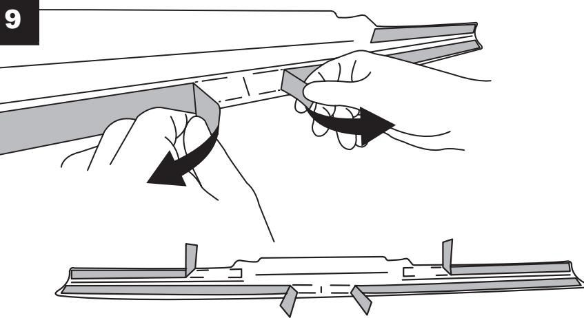
**EN** Peel back approximately 2" in / 50 mm of each inner edges (4) an angle on each side in order to be able to grab them once the spoiler is placed on the roof.
