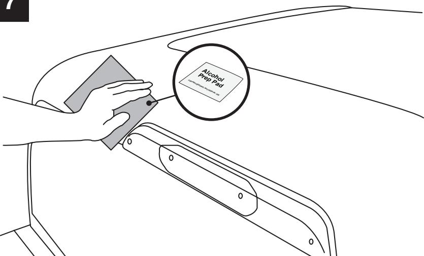
**EN** Using the supplied alcohol pad, clean the area of the roof where the spoiler will be in contact in order to ensure that the surface is clear of all contaminants (Oily film and/or Wax) for a proper installation of the spoiler.
