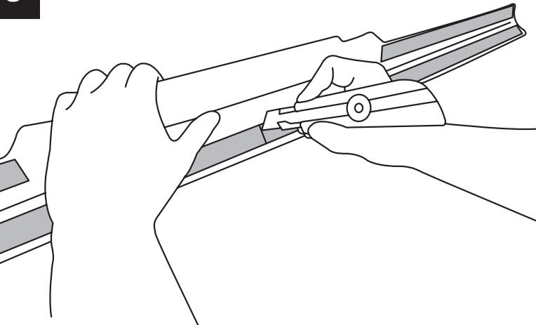
**EN** Carefully cut the front edge, red protective film (liner) at the center, inline with the spoiler top arrow.
