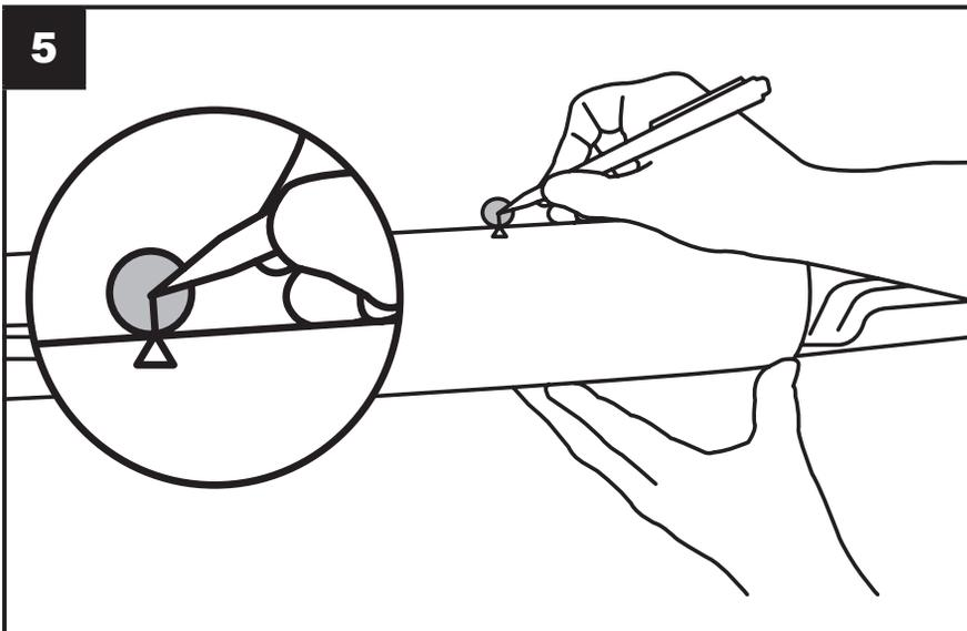
EN While applying pressure on the spoiler, pencil in, a line on the central alignment sticker in line with the arrow at the center of the spoiler to ensure its ultimate reference location during final installation.
