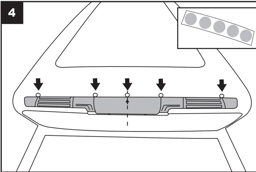
EN While applying pressure on the spoiler, install the 5 alignment stickers to the front edge of the spoiler to mark locations. Starting at the center, aligned with the spoiler's arrow.
