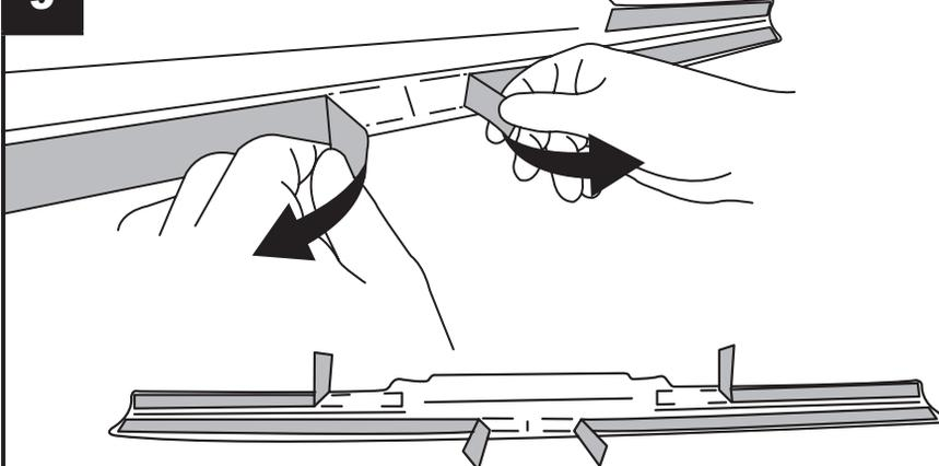
EN Peel back approximately 2" in / 50 mm of each inner edges (4) an angle on each side in order to be able to grab them once the spoiler is placed on the roof.
