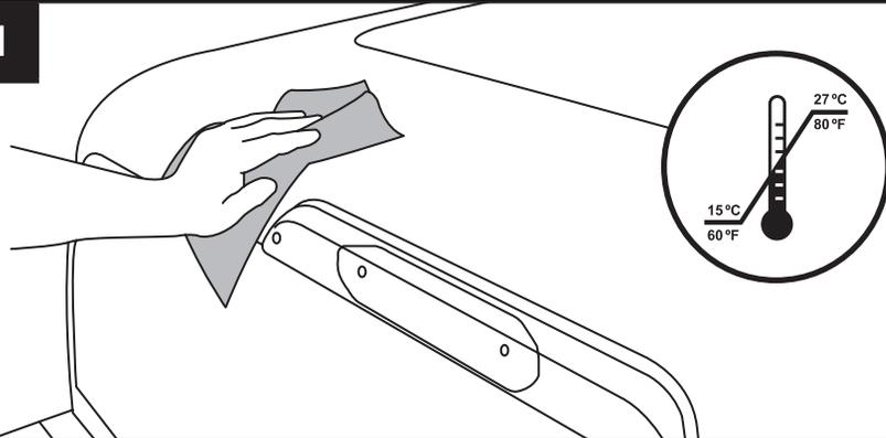
EN Clean the area of the roof where the spoiler will be in contact with the surface using only soap & water and dry with a clean cloth.
