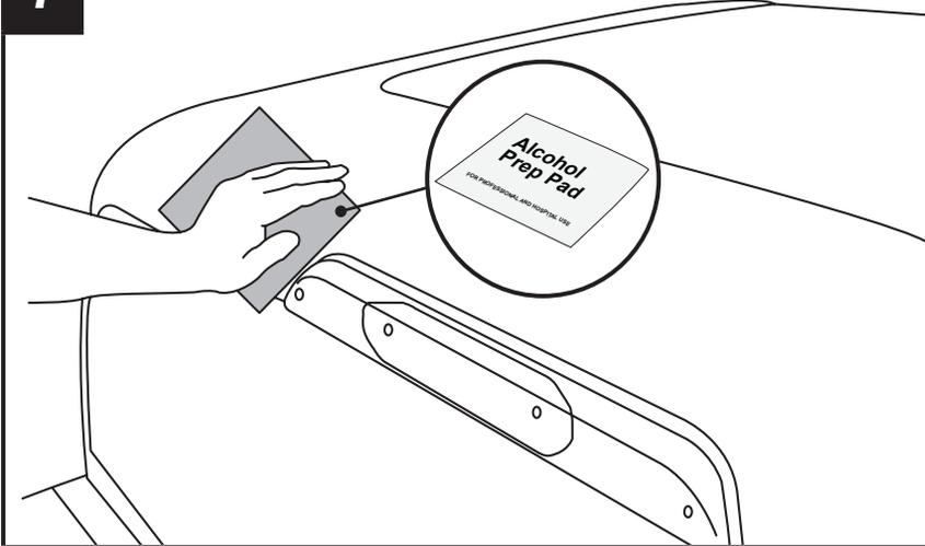
EN Using the supplied alcohol pad, clean the area of the roof where the spoiler will be in contact in order to ensure that the surface is clear of all contaminants (Oily film and/or Wax) for a proper installation of the spoiler.
